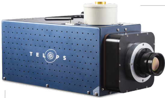
The Telops LN2 camera enclosure
