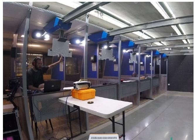
Figure 2. Muzzle flash test environment with Telops FAST M3k camera and shooter position
